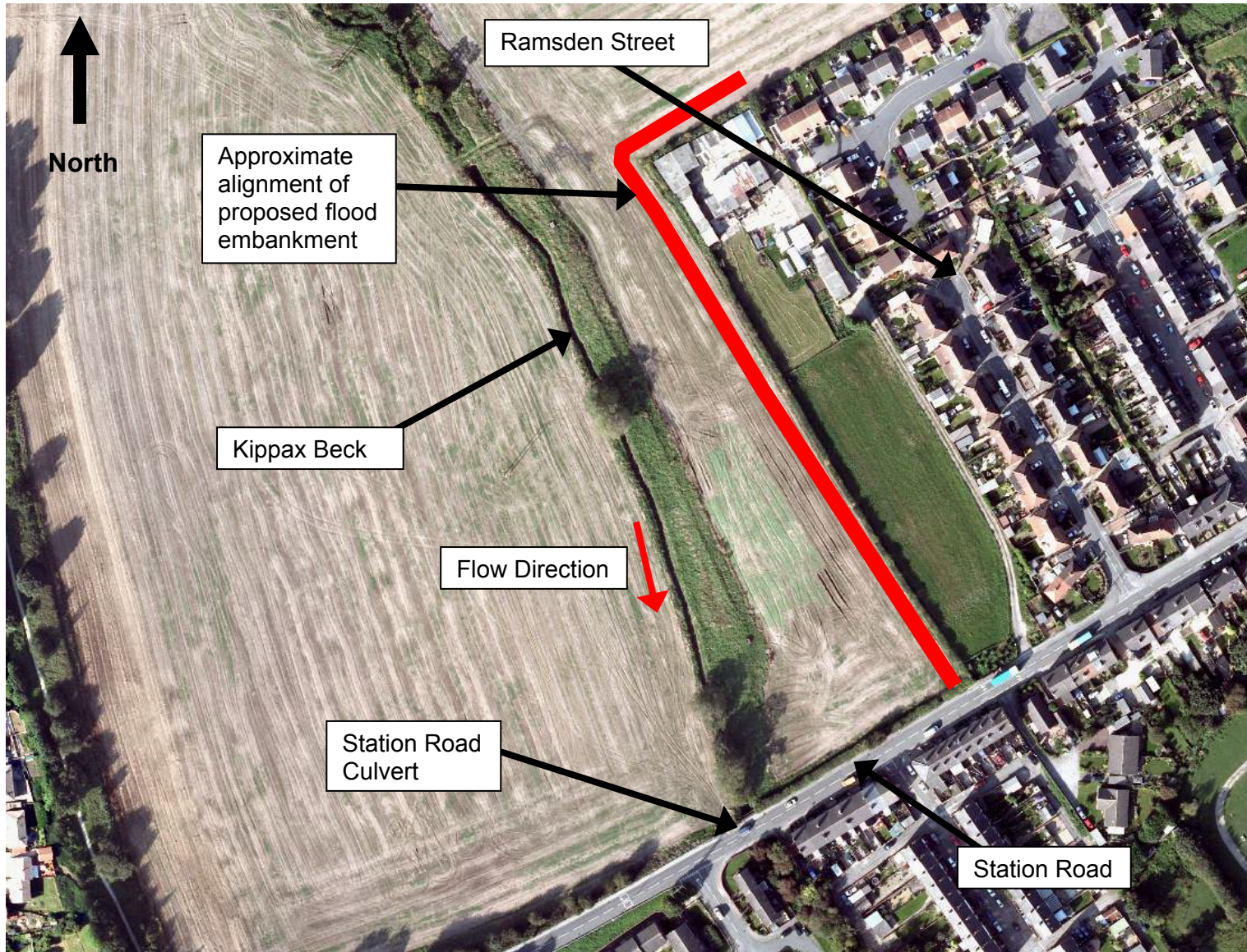
Figure 4 – Approximate alignment of proposed flood embankment
