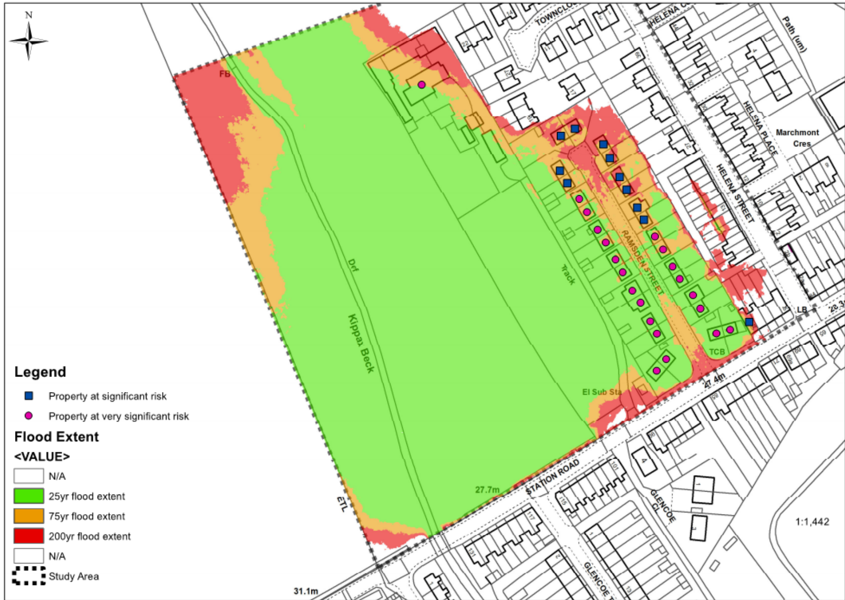
Figure 3 – Properties at risk from flooding at Ramsden Street
